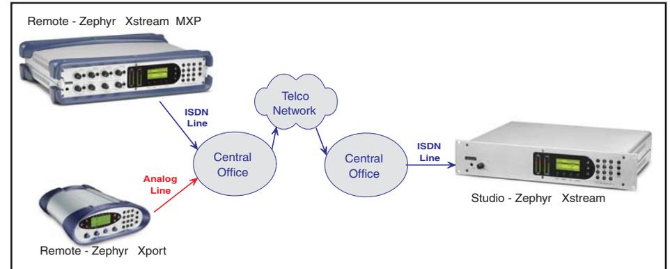
The majority of the public switched telephone network is now completely digital. As the illustration above shows, a POTS call from a Zephyr Xport is converted from analog to digital at the nearest Central Office, where it continues on a digital path all the way to the studio.
