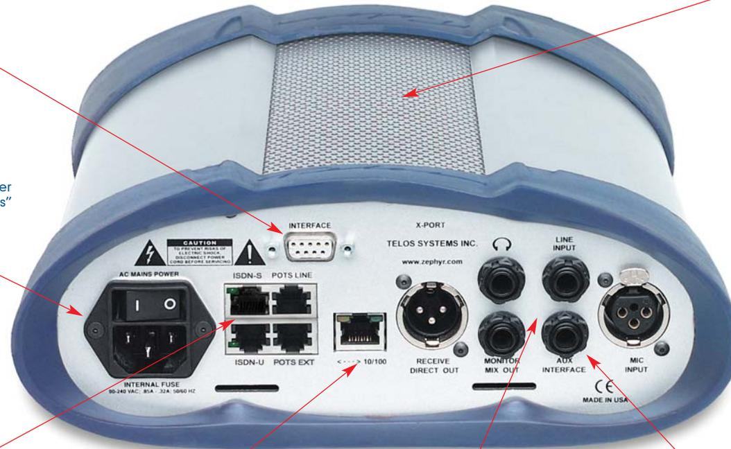
Telephone interface includes connections to an analog (POTS) phone line, a telephone handset for making voice calls, and ports for ISDN connections (when equipped with one of the ISDN transmission options).
