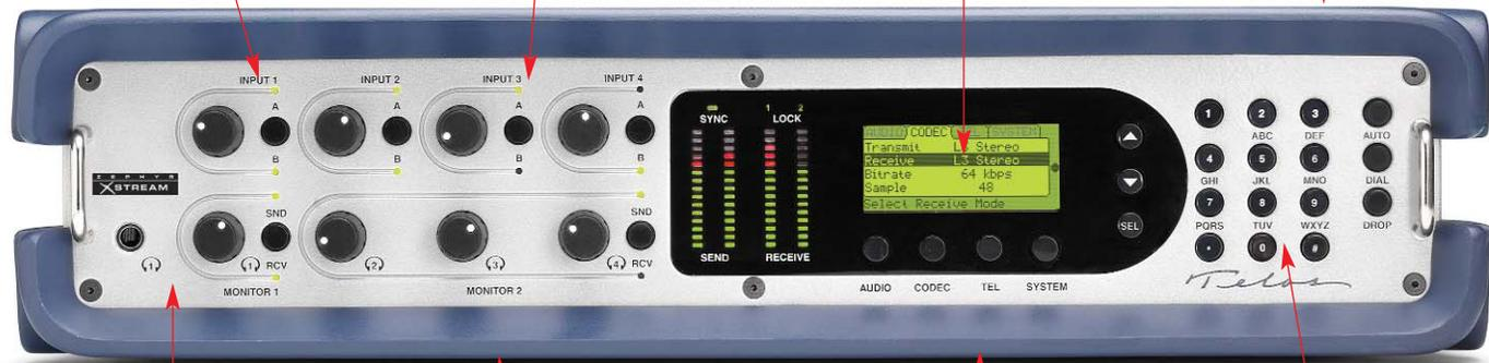
Adjustable front panel headphone jack for Local Mix 1 monitors Send or Receive audio, or a mixture of the two.
