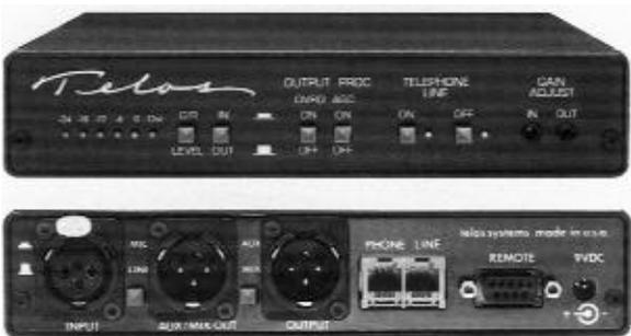
When space or budgets are tight, the modem case version of the Telos ONE is an excellent alternative. Electronically identical to the rack mounting version, it differs only in its enclosure and use of an external power supply.
