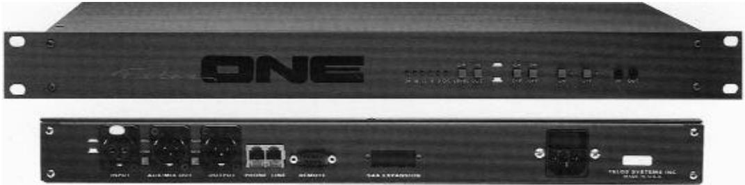
The Telos ONE input may be switched to accommodate either mic or line level. Two outputs are provided, one of which may be switched to provide either an independent caller output or a mix of the input and caller signals. Modular jacks are used for connection of the phone line and, if desired, a
