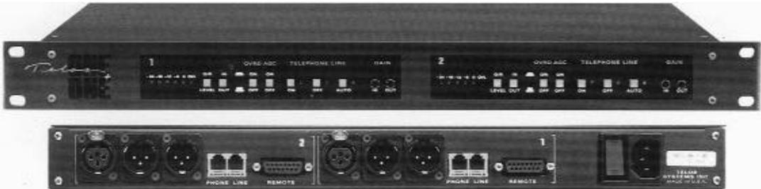
The ONE plus ONE eliminates the need to create complex mix-minus schemes when using two hybrids. Its hybrids may be used independently
